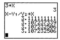
In Derive, load the utility file SOLVE. Enter NEWTON ( $x^3-30$ , x, 3) and then APPROXIMATE to get [3, 3.11111111, 3.10723733, 3.10723250, 3.10723250]. You can request a specific iteration by adding a fourth argument. For example, NEWTON ( $x^3-30$ , x, 3, 2) gives [3, 3.11111111, 3.10723733].
