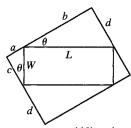
In the small triangle with sides a and c and hypotenuse W,  $\sin \theta = \frac{a}{W}$
