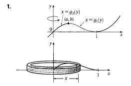
If we were to use the "washer" method, we would first have to locate the local maximum point (a, b) of  $y = x(x - 1)^2$  using the methods of Chapter 4. Then we would have to solve the equation  $y = x(x - 1)^2$  for x in terms of y to obtain the functions  $x = g_1(y)$  and  $x = g_2(y)$  shown in the first figure. This step would be difficult because it involves the cubic formula. Finally we would find the volume using
