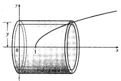
11.  $V = 2\pi \int_0^8 \left[ y(\sqrt[3]{y} - 0) \right] dy$  $= 2\pi \int_0^8 y^{4/3} dy = 2\pi \left[ \frac{3}{7} y^{7/3} \right]_0^8$   $= \frac{6\pi}{7} (8^{7/3}) = \frac{6\pi}{7} (2^7) = \frac{768\pi}{7}$
