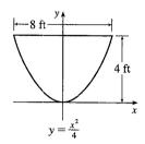
(b) In part (a) we knew the final water level (0) but not the amount of work done. Here we use the same equation, except with the work fixed, and the lower limit of integration (that is, the final water level — call it h) unknown:  $W = 4000 \Leftrightarrow 250\pi \left[2y^2 - \frac{1}{3}y^3\right]_h^4 = 4000 \Leftrightarrow \frac{16}{\pi} = \left[\left(32 - \frac{64}{3}\right) - \left(2h^2 - \frac{1}{3}h^3\right)\right] \Leftrightarrow h^3 - 6h^2 + 32 - \frac{48}{3} = 0.$
